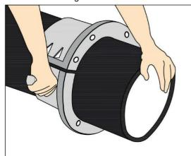
5. Using bolt cutters or a hacksaw, cut the two helix wires flush with the end of the hose. The wire must not protrude out of the hose end.
